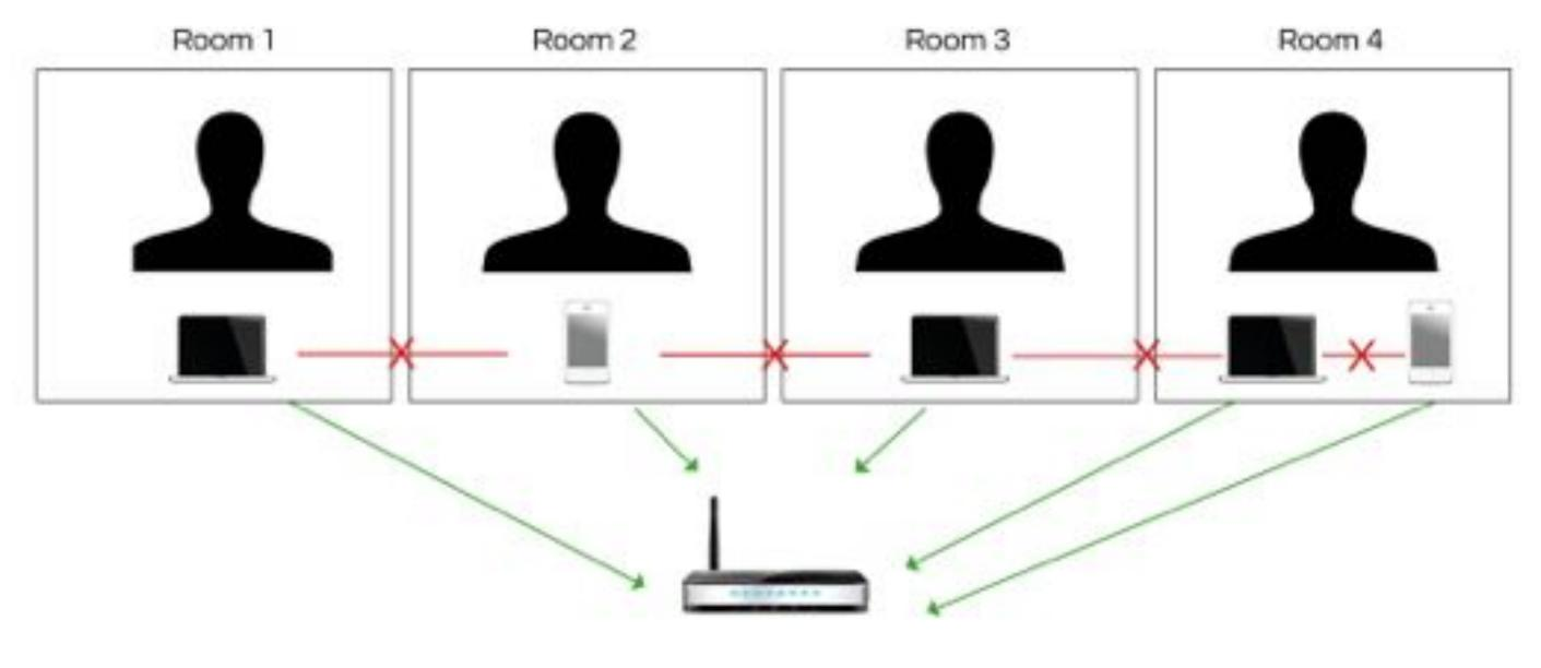
Each device can connect to the outside world vis the HSIA service. But, for security, each device cannot connect with another device.
